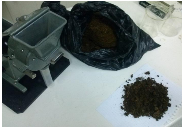
Figure 1: The Material (Sheep Excreta) in The Hammer Mill
